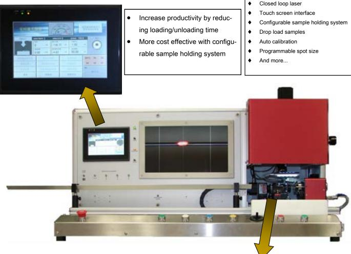
The new configurable drop loading catheter holding system allows fast loading/unloading. Right chuck can be a segmented chuck with 0-1/4" opening, touhy borst or three jaw micro chuck. Air driven adjustable opening catheter clamp on the left. See other configurations on separate page. Adjustable position catheter support trough is standard.
